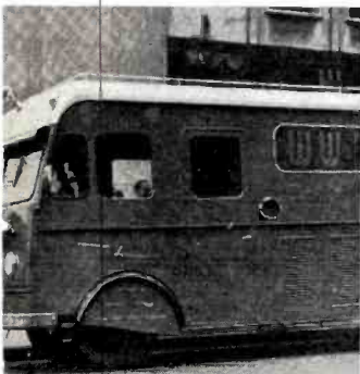
NEW remote truck of WWJ-TV Detroit , custom made to WWJ's specifications by the Ketels Mfg. Co. , was delivered last month and used day following receipt at a baseball telecast from Briggs Stadium . Painted a fire engine red, the truck is 25 ft. long, 9 ft. 6 in. high and 8 ft. wide.
